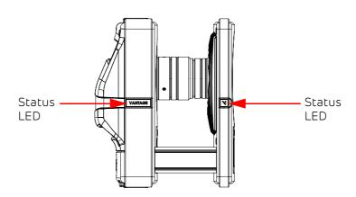
While the camera is booting, the OLED display shows the Vicon logo (unless a connected application causes it to display something else) and the status LED color changes from yellow during booting, to red when booting is complete.
