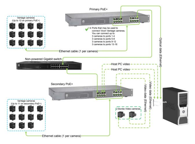
The Bonita video cameras are added to the secondary PoE+ switch so they do not add to the bandwidth of the interconnection to the primary PoE+ switch.
