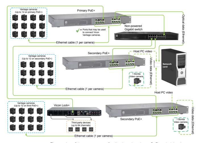
The number of Vantage cameras feeding into the primary PoE+ switch has been 'balanced' by adding a Bonita video camera to each of the secondary PoE+ switches.
