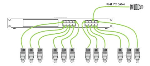
6. Plug the other end of the cable into the PCle network Gigabit Ethernet port for the Vantage system network on the rear of the Vicon Vantage host PC (for details, see Vicon Vantage system network port on page 60).
