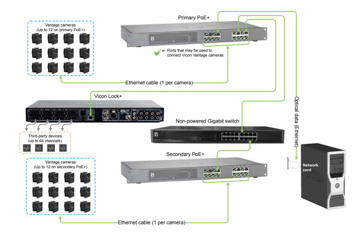
Lock+ is made sync master and is connected directly to the primary PoE+ switch.
