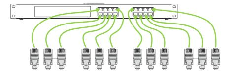
4. Plug the other end of the Ethernet cable (the end with the ferrite) into the RJ-45 socket on the rear of each Vantage camera.
