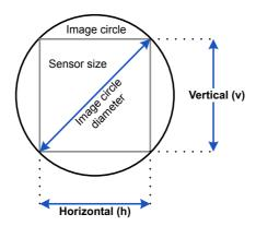
The diameter of this image circle is the maximum area of usable quality image that the lens can produce. Most lenses produce their best image at the center of the lens, dropping off in performance towards the outer extremes of the lens. This results in a gradual darkening towards the edges of the image, known as vignetting. Vignetting gets worse for wider angle lenses and for wider open apertures, but the area at which vignetting starts to occur depends on the lens.
