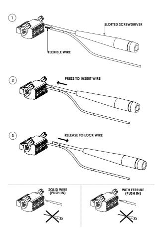
If your cables are rigid (solid wire or ferrule), you do not need to use a screwdriver and can push the ends of the cables into the required connector.
