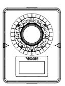
The strobe unit emits a powerful flash of light once per video frame at precisely the same time as the image sensor's global electronic shutter opens. This flash illuminates the retroreflective markers attached to the motion capture subject. The reflected light passes back through the lens and optical filter. The spectral characteristics of the filter ensure that only light with the same wavelength as the LEDs passes back into the camera.
