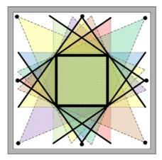
Camera positions will depend on your volume size, camera type, and camera lens. Remember to include height as well as width and depth in your volume calculations.
