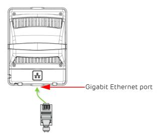
The following single connection point is beneath the rear panel:
