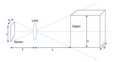
The sensor area used for capturing data through each Vicon Vantage camera determines the maximum FOV available for a particular combination of camera and lens. The area of the sensor is determined by its horizontal width (h) and vertical height (v).
