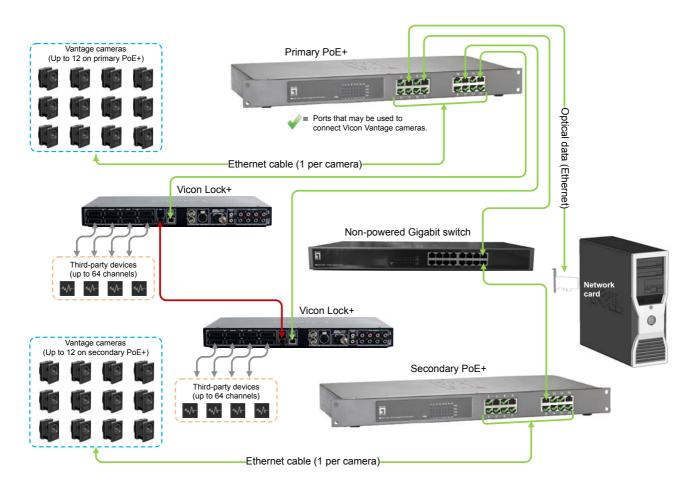
Two Lock+ units are added to the primary PoE+ switch. Connecting a genlock source such as Reference Video In or VESA Stereo In will determine which Lock+ is sync master. If both sources are to be used, connect them both to the same Lock+.
